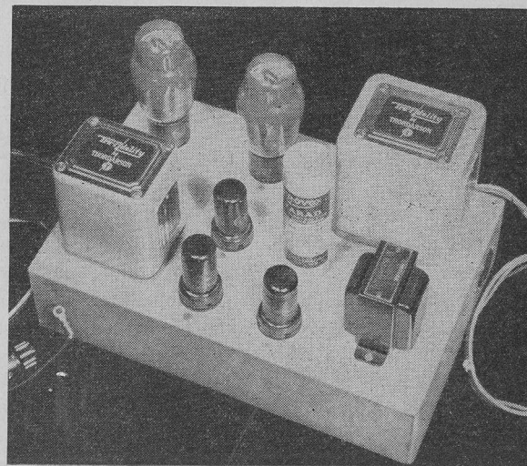
Fig. 45—Appearance of the finished transformer-coupled amplifier.
